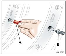
'R' performance wheels – These wheels have a slotted valve cover on the wheel face. A pouch containing a special tool and a valve adaptor, for use with these wheels, is stowed in the glove compartment.
