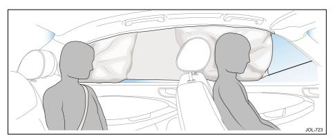
When the curtain airbag inflates upon a vehicle side impact, it breaks through the headlining and deploys downwards, giving head protection to front and rear seat occupants.
