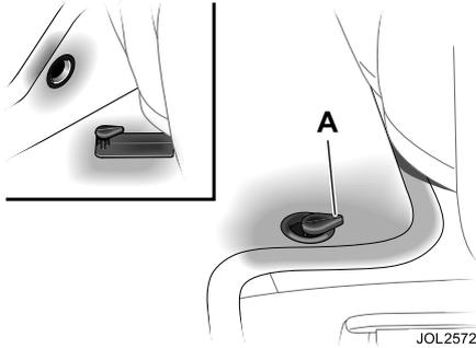
Ensure that the driver's floor mat is correctly positioned and secured under the tongues on the retention posts (A, only one post shown), so that the mat does not interfere with the operation of the accelerator, clutch or brake pedals. In particular, check the position of the mat when refitting after cleaning or servicing.
