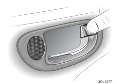
To centrally lock all doors, press the lock lever on the driver's or front passenger's door.
