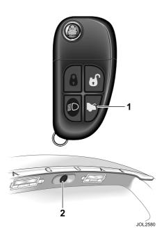
If the vehicle alarm system is armed and the luggage compartment is opened using the key transmitter the alarm will not sound. The system will be rearmed when the lid is closed, provided the vehicle has not been disarmed.
