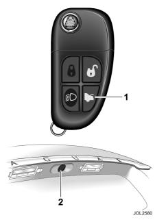
If the vehicle alarm system is armed and the luggage compartment is opened using the key transmitter the alarm will not sound. The system will be rearmed when the lid is closed, provided the vehicle has not been disarmed.
