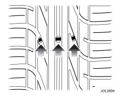
It should be noted that the properties of many tyres alter progressively with wear. In particular the 'wet grip' and aquaplaning resistance are gradually but substantially reduced. Extra care and speed restriction should therefore be exercised on wet roads as the effective tread depth diminishes.
