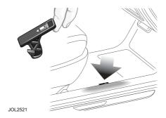
Pull the fuel filler flap release. This is located on the floor, outboard of the driver's seat, see page 127.
