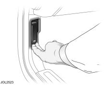
Pull the release lever located below the fascia on the left-hand side of the vehicle, see page 169.
