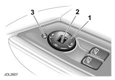
Both door mirrors are adjusted from the driver's door switchpack. The four-way adjustment button (1) moves the mirrors to the required position. The selector switch (2) selects the mirror to be moved, left for the left-hand side mirror and right for the right-hand side mirror. When the selector switch is in the centre position, adjustment to either mirror is inhibited.
