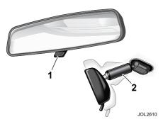
Interior mirrors are either manual dip or electrochromic.
