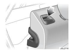
**Estate:** Release catches are located on the top of each seat back. Press the catch to release the seat back.
