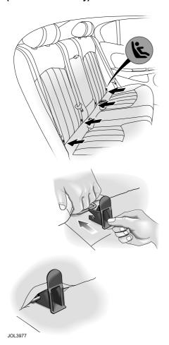
Only the Britax Roemer Duo Plus ISOFIX restraint is approved by Jaguar for use with this system. An ISOFIX anchorage kit must be fitted to your vehicle before the ISOFIX seat can be installed. These brackets must be supplied and fitted by your Jaguar Dealer/Authorised Repairer. The ISOFIX anchorage kit and the ISOFIX seat cannot be installed in Estate models. The ISOFIX system allows an ISOFIX child.
