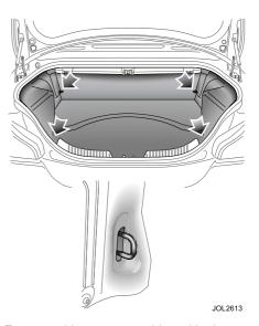
Four metal loops are positioned in the luggage compartment for attaching straps to secure loads and prevent them from sliding over the luggage floor.
