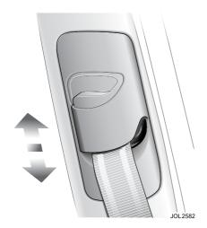
**To operate:** Press the locking button and slide the anchorage point to the required position to ensure comfort and safety. Release the button and check that the anchorage point is locked.
