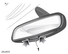
Push the switch (1) in and the electrochromic rear view mirror darkens automatically to prevent glare from a following vehicle's headlights. The mirror clears when light levels return to normal. The mirror also clears when reverse gear is selected.
