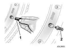
These wheels have a slotted valve cover on the wheel face. A pouch containing a special tool and a valve adaptor, for use with these wheels, is stowed in the glove compartment.
