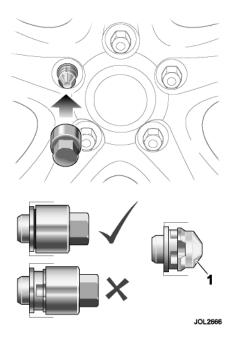
Where Jaguar locking wheel nuts are fitted (one on each wheel), they can only be removed using the correct key socket.
