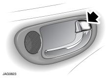
To lock all doors centrally, press the lock lever on either the driver's or the front passenger's door.
