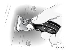
Child safety locks are fitted to the rear doors. Open a rear door, insert the starter key into the lock and turn the key towards the outside of the vehicle. This immobilises that door interior handle. Repeat this for the opposite rear door. After setting the child lock the door(s) can only be opened using the exterior door handle.
