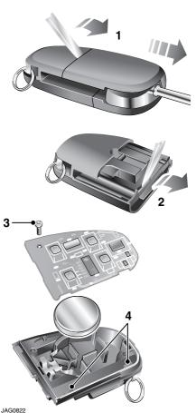
When the battery needs renewal there will be a significant decrease in the effective range of the key transmitter. To renew the battery, follow the procedure below:
