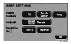
After touching the **User Settings** button, the screen displays the buttons for the selection of audible feedback, language, and units of measurement.
