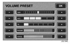
After touching the **Volume** button, the screen displays the buttons for adjustment of volume associated with the navigation system, Jaguar Voice, telephone, Traffic
