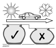
A colder ambient local temperature will reduce pressure within the tyre. An effect is to decrease sidewall height and to increase tyre shoulder wear with the potential for tyre failure. Vehicle dynamics could also be adversely affected.
