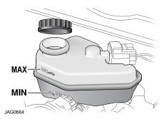
The manual transmission clutch fluid is shared with the brake fluid in a common reservoir.
