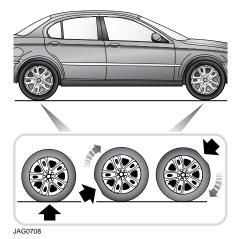
This is normal tyre behaviour, however, when the vehicle is subsequently driven, vibration may be experienced from the flat spot. The condition will steadily improve with additional mileage.
