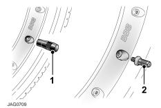
These wheels have a slotted valve cover on the wheel face. A pouch containing a special tool and a valve adaptor, for use with these wheels, is stowed in the glove compartment.
